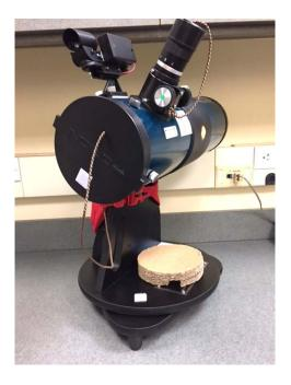
Replace the cardboard disc under the Optical Tube Assembly...
